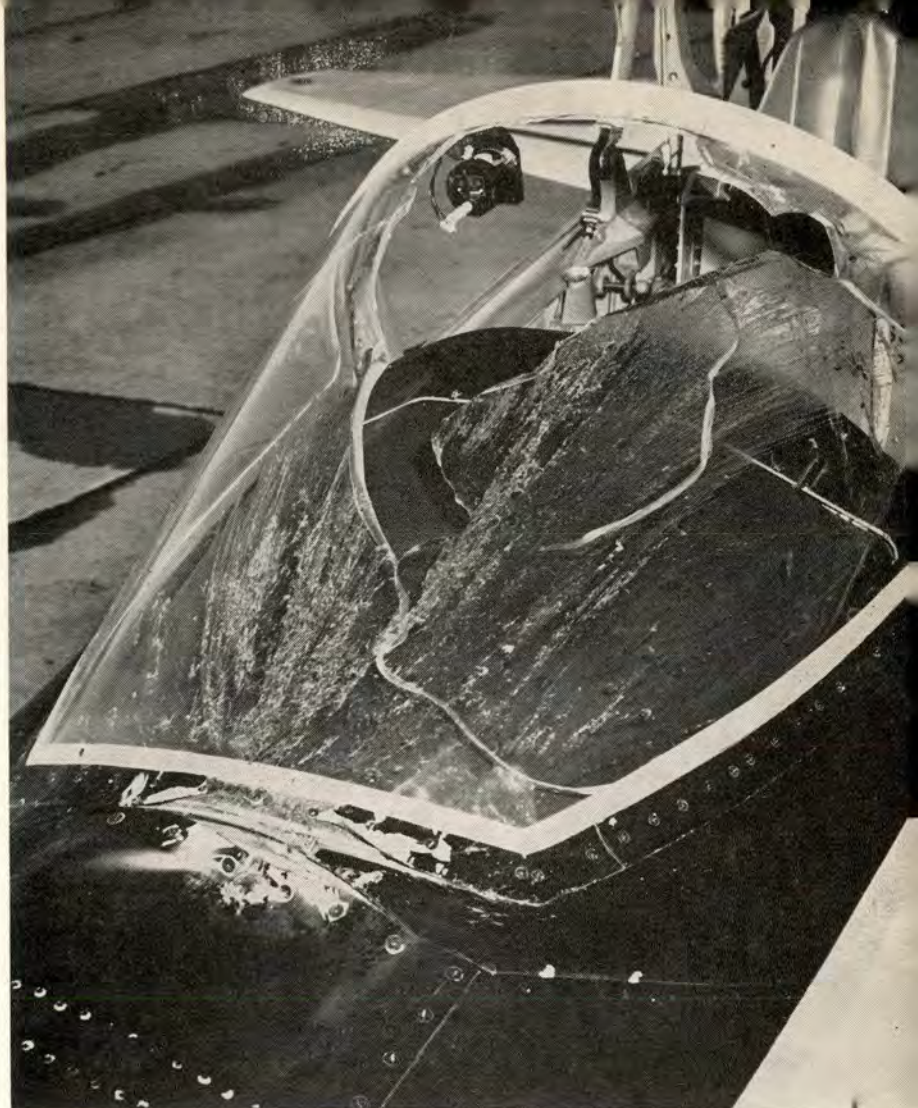
This is what happened when a 3-lb duck and the windshield of a T-38 collided. Bird did not enter cockpit, but residue was found on student pilot's visor, which was down.
